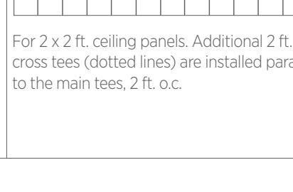
For 2 x 2 ft. ceiling panels. Additional 2 ft. cross tees (dotted lines) are installed parallel to the main tees, 2 ft. o.c.
